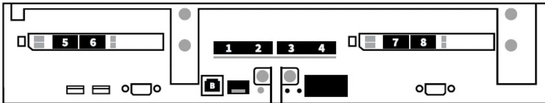
Figure 5. Recommended DGX H100 system network port connections.
